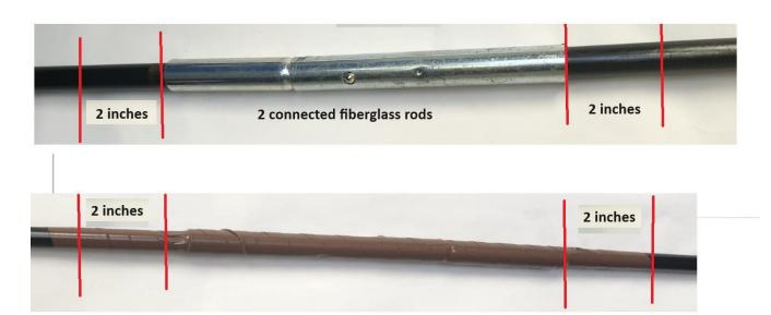
Tape over both fitting as shown on the photo. Tape 2 inches pass each fitting on the left and right side. Tape about 5-6 layers and make sure its tight. Repeat this process at every silver junction. Not Taping properly will cause the net pole to drop and cause damage to the net and fiberglass rod and will not be covered under warranty.
